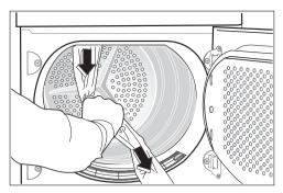
3. Remove foil hose and polystyrene padding from the machine.
